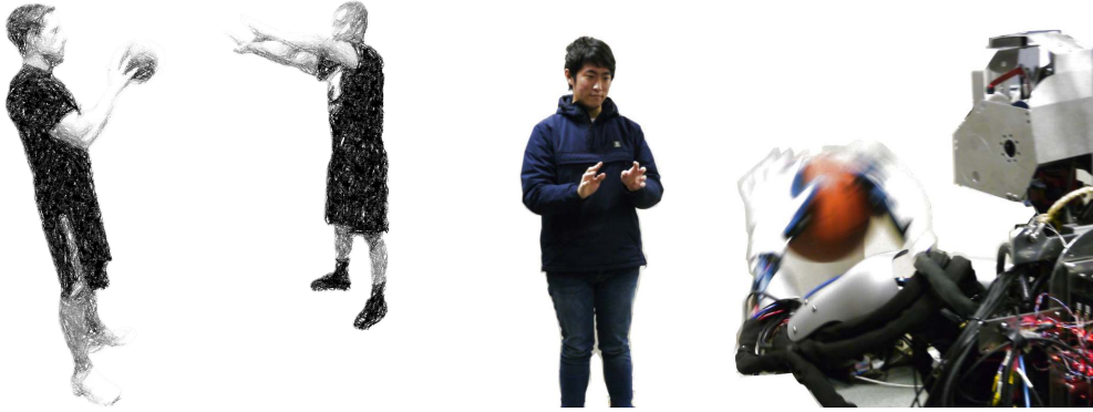
Figure 1: Playing with a ball. Humans are naturally endowed with the ability to estimate the time-to-contact while coordinating multiple degrees of freedom even without knowing the exact dynamics of the flight of the ball and the involved contact forces. To endow robots with such capabilities, this article introduces Phase Portrait Movement Primitives (PPMPs). A PPMP is capable of estimating the future temporal states of an interaction by using coupled oscillators as a low-dimensional dynamical model in phase space. By using policy search, the robot learns to combine the estimated phase with the high-dimensional kinematics of the task represented as a phase portrait.
