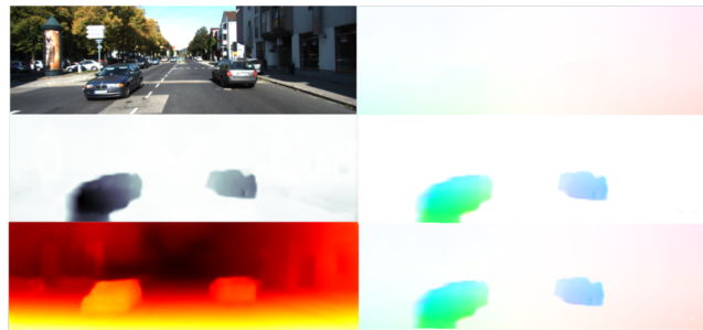
Figure 1: Unsupervised Learning of Depth, Camera Motion, Optical Flow and Motion Segmentation. Left, top to bottom: sample image, soft masks representing motion segmentation, estimated depth map. Right, top to bottom: static scene optical flow, segmented flow in the moving regions and combined optical flow.
