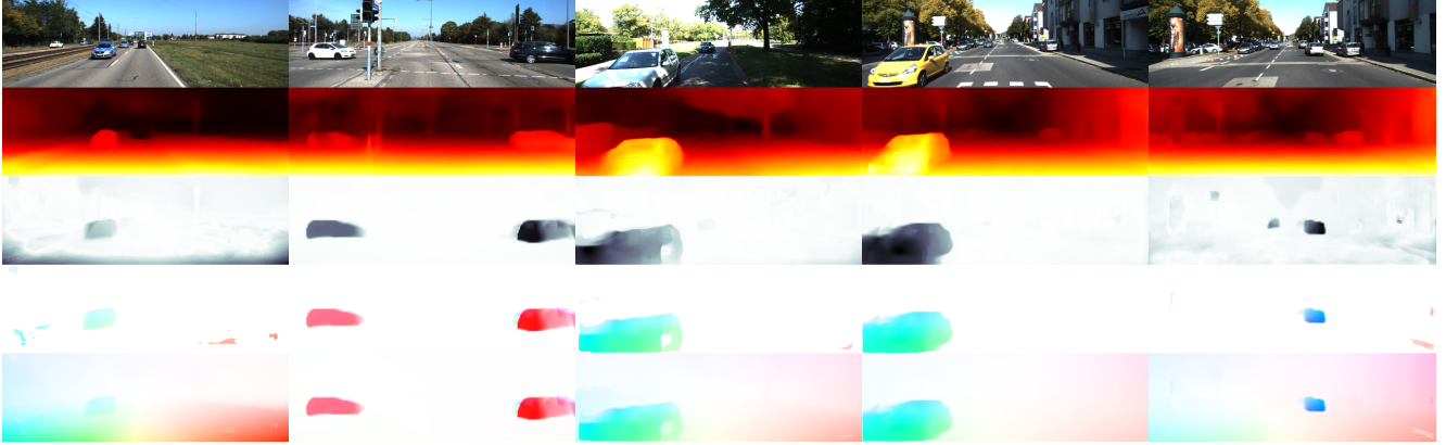
Figure 4: Visual results. Top to bottom: Sample image, estimated depth, soft consensus masks, motion segmented optical flow and combined optical flow.
