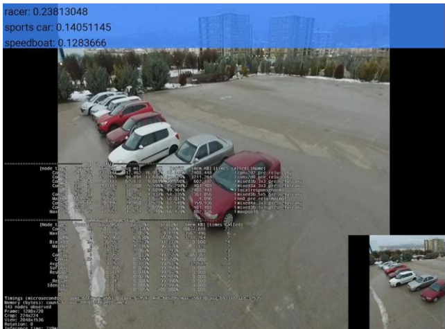
Fig. 9 Classification Activity Vehicle Detection with Details Layer Activated (UAV Hovering Over Ankara University Computer Engineering Department Parking Lot)
