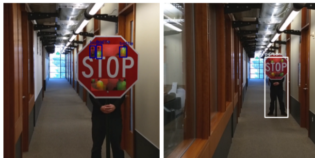
Figure 3: YOLO detection output for a real stop sign with adversarial stickers (still frames from video)
