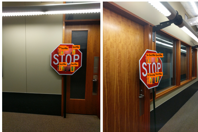
Figure 2: YOLO detection output for a real stop sign with adversarial stickers (phone camera pictures)
