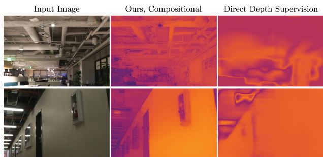
Figure 7. A qualitative comparison of monocular depth estimation results from the test set of our DSLR dataset experiments. Our aperture supervision model is able to estimate more detailed depth maps than the direct depth supervision baseline.
