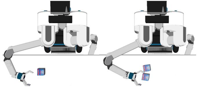
(a) Two states with object pose that differs by less than 1cm (b) After executing the same action, the final object pose differs significantly.
