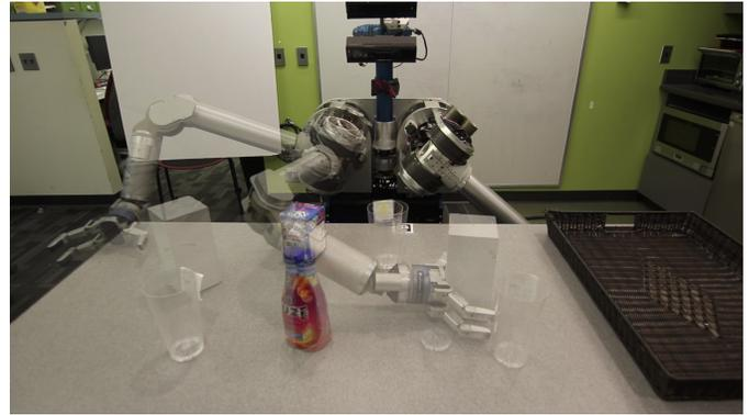
Fig. 1: A solution to a rearrangement problem. The robot moves the box across the table to make it reachable by the left arm. The robot freely interacts with and moves clutter in the scene in order to achieve the goal.
