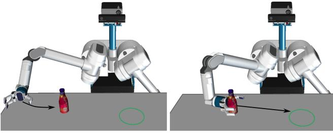
(a) The *contact* primitive tries to make contact between the palm and the goal object. (b) The *pushing* primitive moves the end-effector in the direction of the goal region
