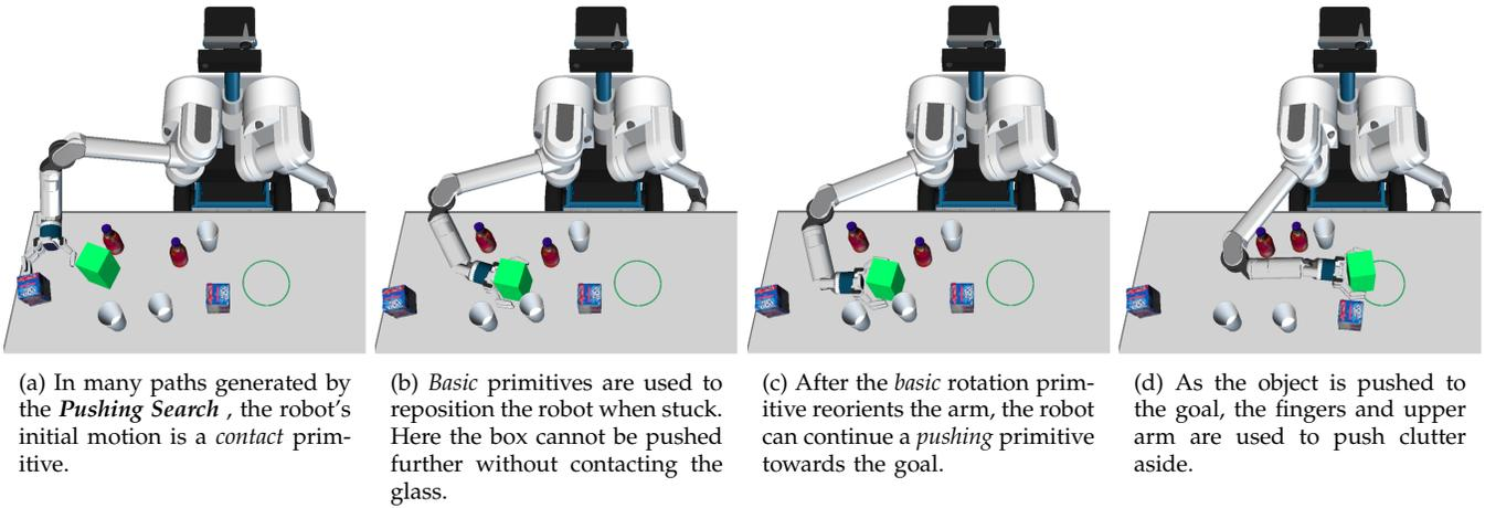
Fig. 6: A solution for one of the 12 simulation scenes. The robot is tasked with pushing the green box into the green circle.
