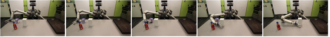
Fig. 2: A rearrangement planning problem. The robot is tasked with pushing the white box near the tray. The plan exhibits *contact* and *pushing* primitives to move clutter and achieve the goal.
