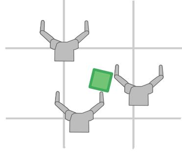
Fig. 3: A simple example of a hand pushing objects. The *basic* primitives allow the hand to translate along the grid lines. In this simple example, the object is “trapped”, i.e. there are no primitives that allow it to move out of the cell.
