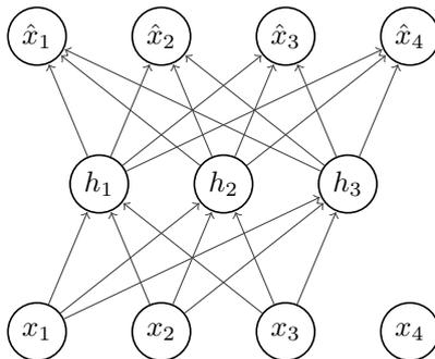
Figure 4.2: Architecture of a NADE with 4 input variables and 3 hidden units. Its input variables are  $x_1, x_2, x_3$  and  $x_4$  (bottom layer), its hidden units are  $h_1, h_2$  and  $h_3$  (middle layer) and its outputs are  $\hat{x}_1, \hat{x}_2, \hat{x}_3$  and  $\hat{x}_4$  (top layer). Note that input  $x_4$  is not actually forward-propagated, thus there are no connections from it to the hidden units.
