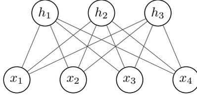
Figure 4.1: Graphical model of an RBM with 4 visible and 3 hidden variables. Its visible variables are  $x_1$ ,  $x_2$ ,  $x_3$  and  $x_4$  (bottom layer) and its hidden variables are  $h_1$ ,  $h_2$  and  $h_3$  (top layer).
