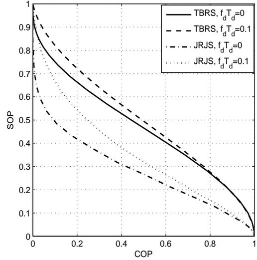
Fig. 3. SOP versus COP for the TBRs and JRJS strategies with different feedback delays for  $N_t = K_r = 3$ ,  $R_s = R_0/8$ , and  $\lambda = 1/10$ .
