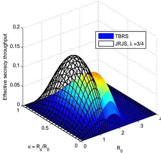
Fig. 8. Secrecy throughput versus  $R_0$  and  $\kappa = R_s/R_0$  for both the TBRS and JRJS strategy with  $N_t = K_r = 3$ ,  $f_d T_d = 0.1$  and  $\eta = 15\text{dB}$ .
