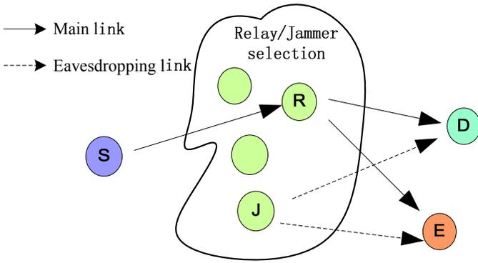
Fig. 1. A cooperative relaying network assisted by multiple relays in the presence of an eavesdropper.
