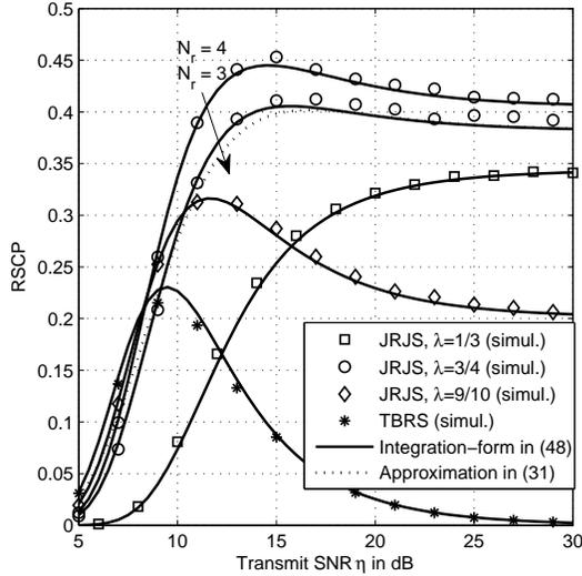
Fig. 5. RSCP versus transmit SNR for the JRJS strategy for different power sharing ratios  $\lambda$  as well as for  $N_t = K_r = 3$ ,  $f_d T_d = 0.1$ , and  $R_0 = 1$ ,  $R_s = R_0/8$ .
