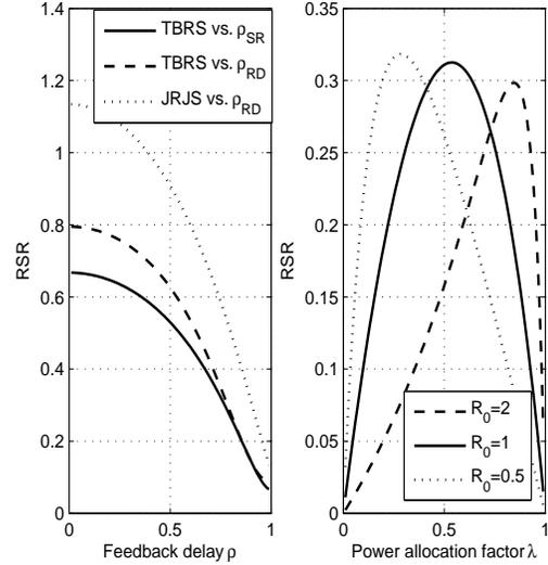
Fig. 6. RSR versus feedback delay coefficient ( $R_0 = 1$ ,  $R_s = R_0/8$ ,  $\lambda = 3/4$ ) and power sharing ratio ( $R_s = R_0/8$ ,  $\rho_{SR} = \rho_{RD} = 0.9$ ) for TBRs and JRJS strategy with  $N_t = K_r = 3$ .
