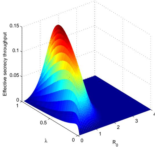
Fig. 9. Secrecy throughput versus  $R_0$  and  $\lambda$  for the JRJS strategy with  $N_t = K_r = 3$ ,  $f_d T_d = 0.1$ ,  $\eta = 15\text{dB}$  and  $R_s/R_0 = 1/8$ .
