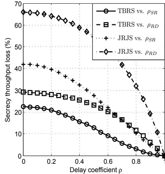
Fig. 7. Percentage secrecy throughput loss versus delay coefficients with  $N_t = K_r = 3$ ,  $R_0 = 1$ ,  $R_s = R_0/8$ ,  $\lambda = 3/4$  and  $\eta = 10\text{dB}$ .
