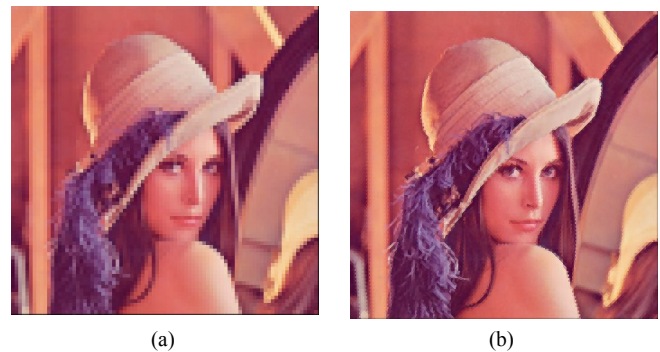
Fig. 1. An image represented using (a) square pixel layout and (b) variable pixel layout.
