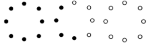
Figure 2. Examples of LBP operators. A solid circle means the pixel is darker than the central pixel. A hollow one means the opposite
