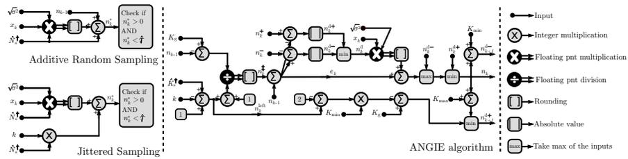
Figure 5: Block diagram showing the generation of one sampling point in the Additive Random Sampling, the Jittered Sampling and the ANGIE algorithm.
