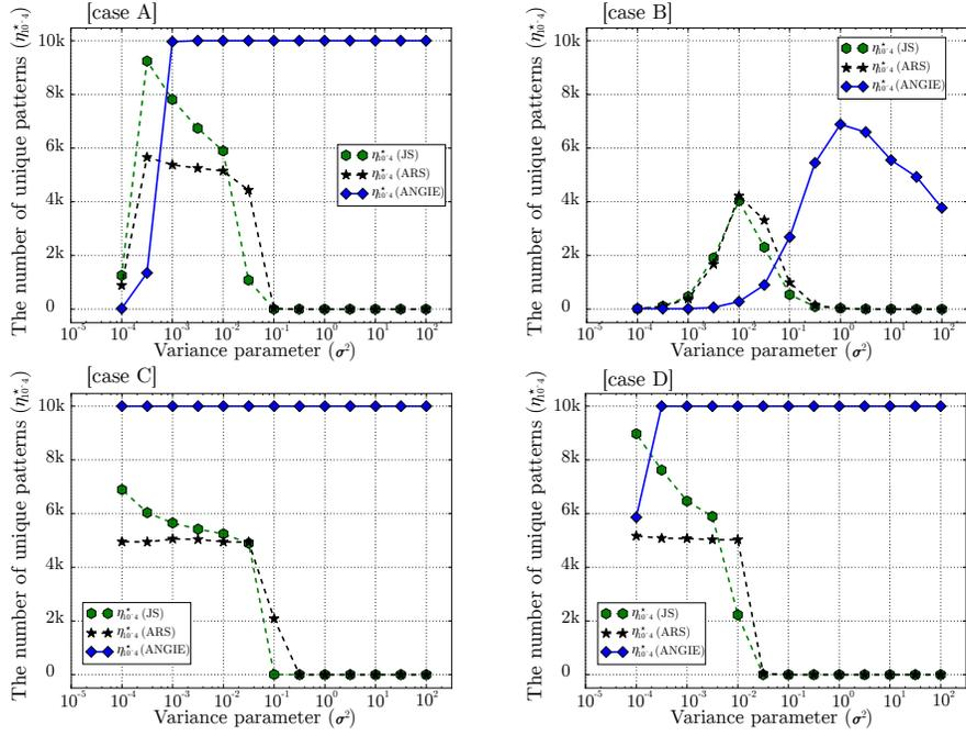
Figure 13: The number of unique patterns  $\eta_{10^4}^*$  (parameter computed for correct patterns only) computed for patterns generated by the JS, ARS and ANGIE algorithms in all the four cases of the experiment #2.
