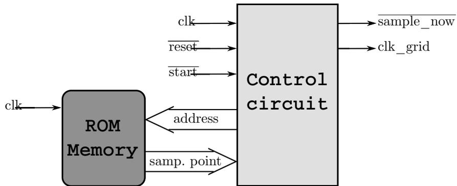
Figure 16: Block diagram of an implemented ADC driver.
