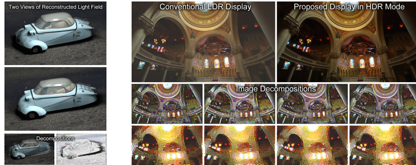
Fig. 3. Left: Compressive light field display mode. We can use the algorithm by Lanman et al. [3] to generate low-rank glasses-free 3D content with the diffuser switched off. Simulated here is a rank-8 light field that has 5 \times 3 views. On the bottom we show a single time frame for both the front and the rear liquid crystal panel. Right: High dynamic range display mode. The diffuser is switched off and a light field with no angular variation, but a higher contrast than that of the LCD panels is emitted. With a simulated black level of 15%, a conventional display only achieves a low dynamic range (top left) whereas the proposed dual layer display (4-frame time-multiplexed here) significantly increases the dynamic range for 2D image display (top right).
