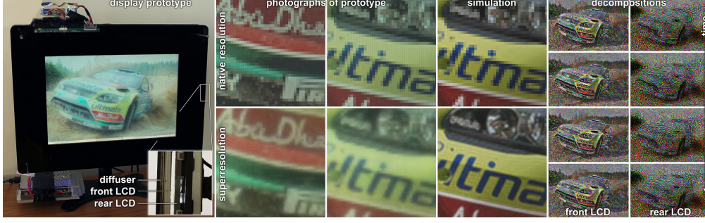
Fig. 1. Compressive superresolution display. The proposed display architecture comprises two stacked high-speed liquid crystal displays (LCDs) covered by a diffuser (left). A target high-resolution image is then decomposed into a set of patterns that are shown on the front and rear LCD in quick succession (right). Compared to the native resolution of each panel (center, top row), the proposed compressive display approach achieves significant improvements in resolution (center, bottom row) without any mechanically moving parts. Display content under CC license: LINK
