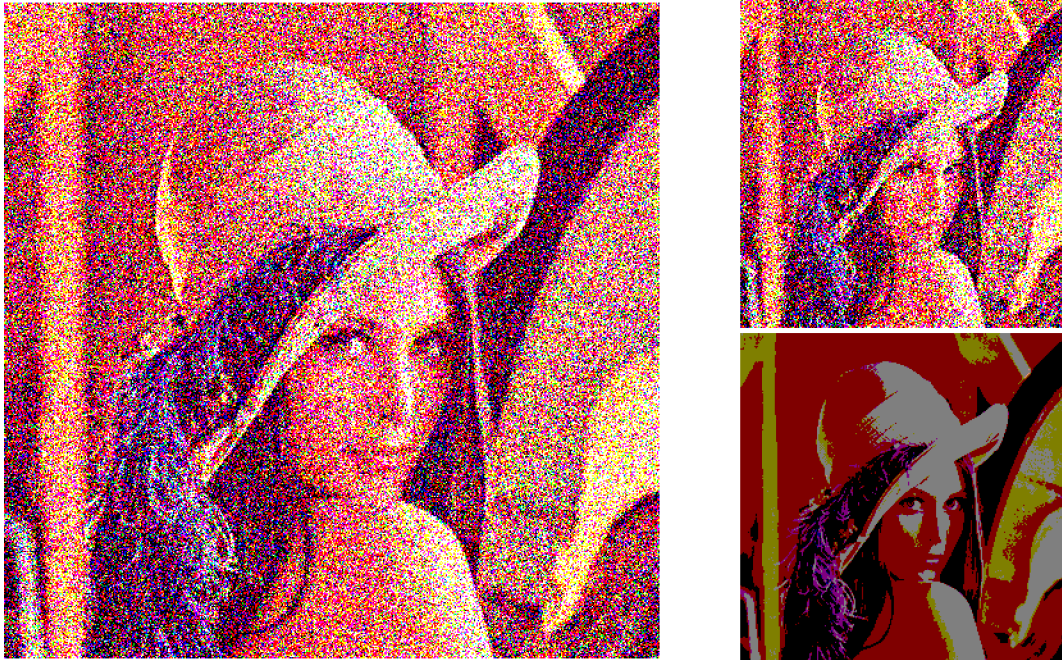
Figure 6: Examples of 3bit/pixel color analogs of Fig. 1 - this time levels of three basic colors of RGB picture are treated independently as they would be grayscale levels. The visual aspect also reduces the rate to about 0.83, so the left code may contain about 79kB of 96kB required to write it - storing halftone picture alone costs about 18kB (Section 7).
