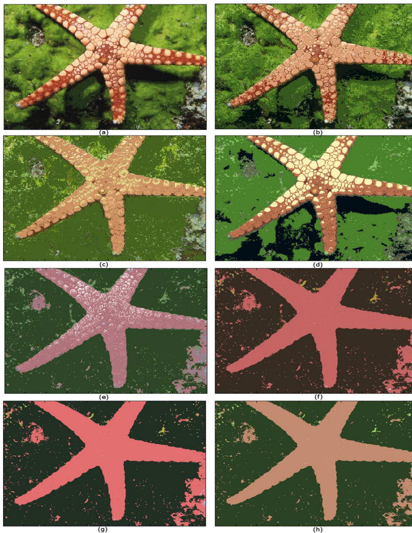
Fig. 1. A random sequence of Starfish Image segmented via unsupervised conformal learning algorithm. (\mathcal{C}_p, \text{NoClust}, \text{TRErr}) represent the tuple containing the Chebyshev parameter ( \mathcal{C}_p ), number of clusters generated (NoClust) while using \mathcal{C}_p and the total reconstruction error of the generated image from the original image (TR-Err)(a) (3, 1034, 17.746), (b) (5, 271, 36.32), (c) (7, 159, 54.71), (d) (9, 45, 40.591), (e) (11, 31, 62.606), (f) (13, 29, 66.061), (g) (15, 33, 65.424), (h) (17, 24, 64.98).
